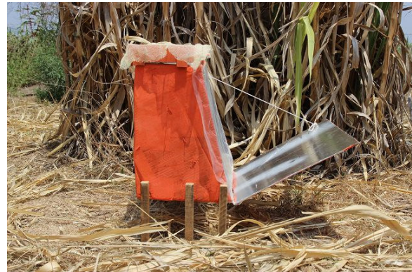
Side view of the finished solar dryer.
